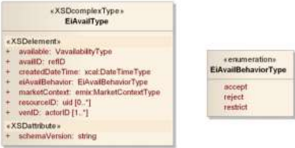
1875 1876 Figure 11-2: UML Class Diagram for the EiAvail Type 1877
