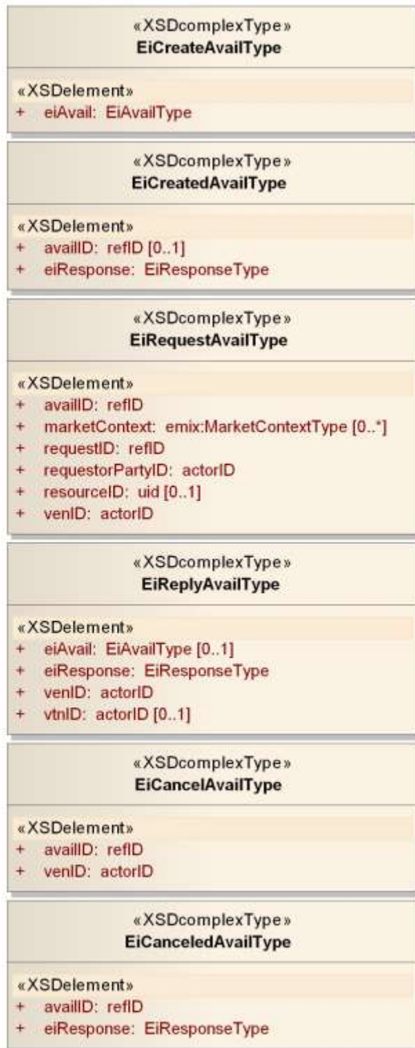
Figure 11-3: UML Class Diagram for EiAvail Service Operation Payloads
