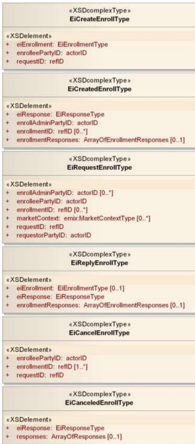
Figure 8-4: UML Class Diagram for Enrollment Payloads
