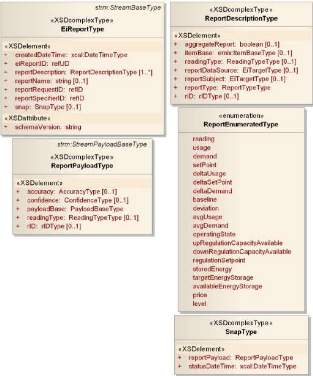
Figure 5-16: UML Class Diagram of Reports
