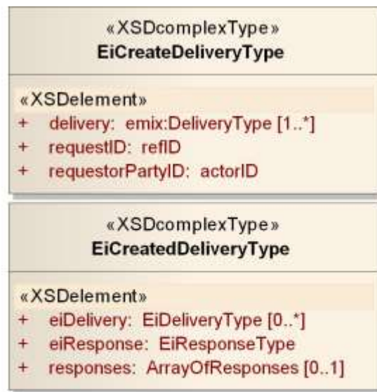
Figure 7-12: UML Class Diagram of Delivery and Delivery Payload
