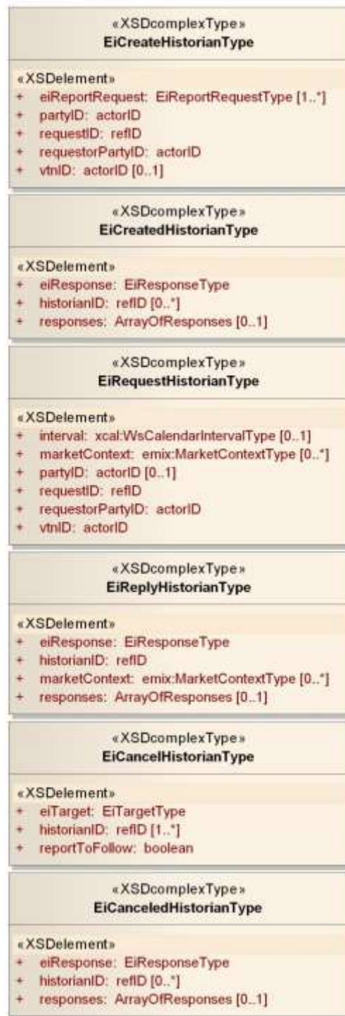
Figure 10-2: UML Diagram of Historian Payloads
