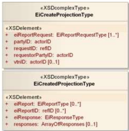
1813 1814 Figure 10-7: UML Diagram of Projection Payloads
