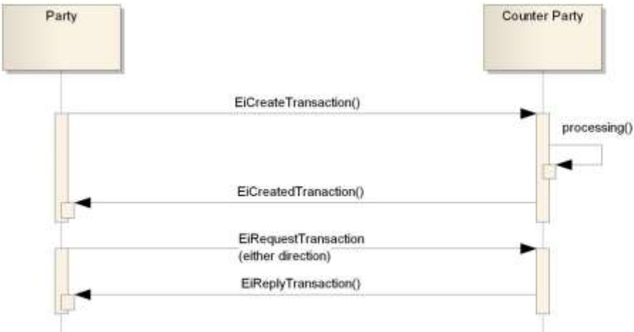
1579 1580 Figure 7-8: Interaction Diagram for the EiTransaction Service
