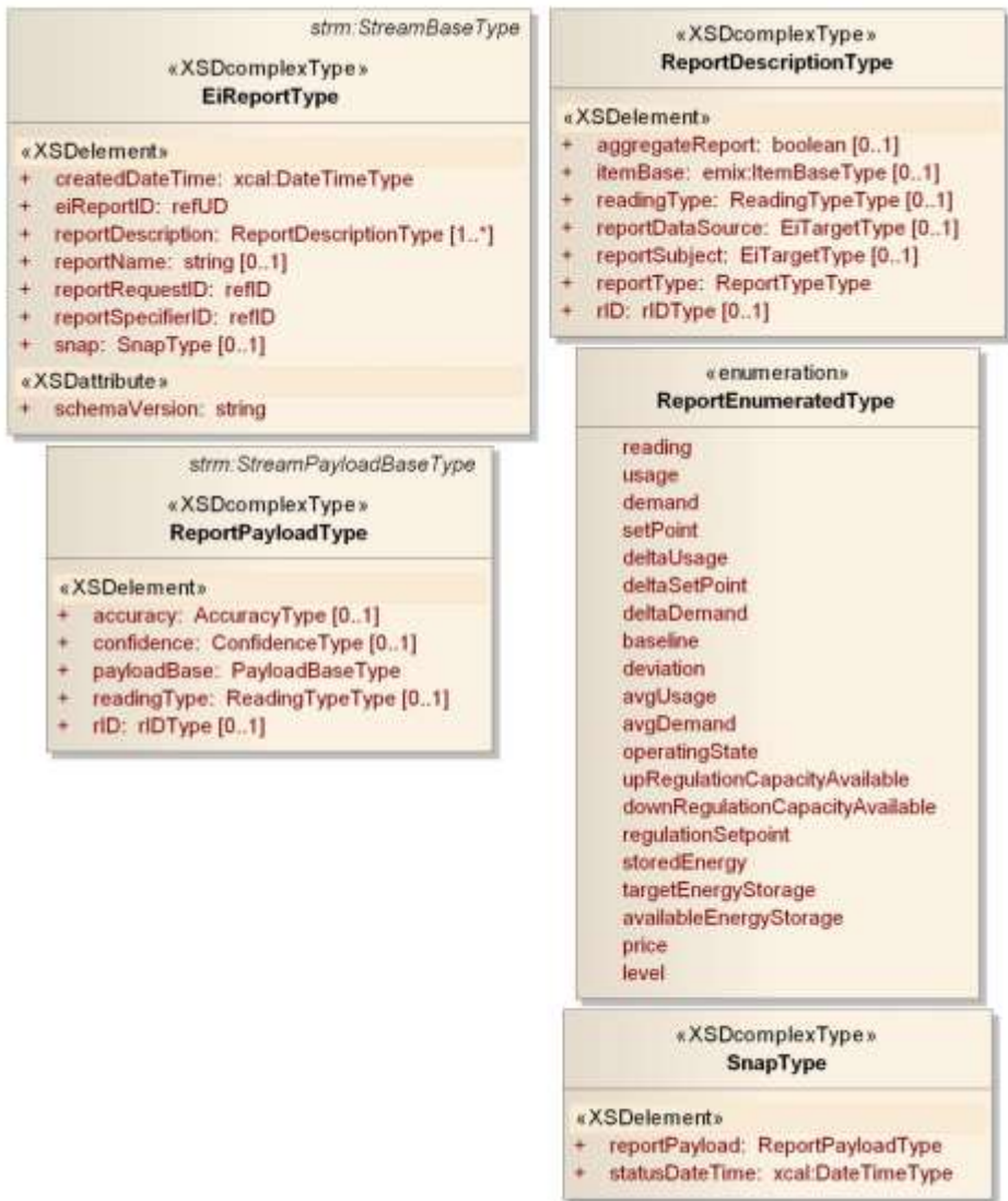
1795 1796 Figure 10-3: UML Class Diagram for the EiReport Class 1797
